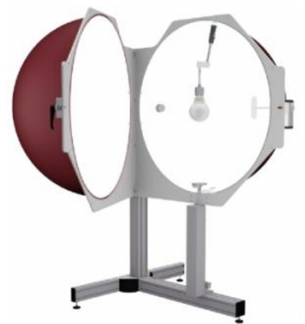
BTS256-LED with an optional 100 cm diameter integrating sphere that has a sample holder for 4\pi lamps.
