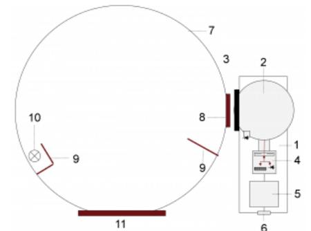
*1) BTS256-LED 2) 50mm integrating sphere 3) Precision bayonet mount 4) BiTec sensor with Si photodiode, CMOS diode array spectrometer and shutter 5) Microprocessor 6) USB interface 7) ISD-21 integrating sphere 8) Bayonet mount 9) Baffle 10) Auxiliary lamp 11) Measurement port*
