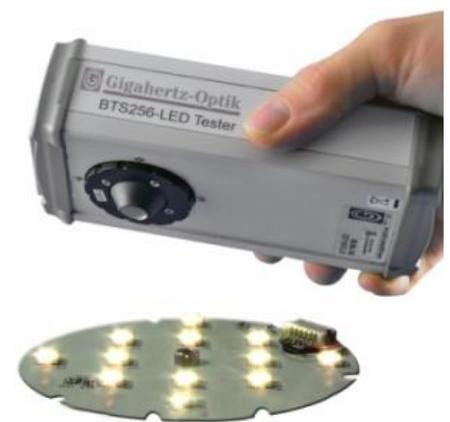
*BTS256-LED for measurement of the*
