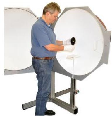
*BTS256-LED Tester with 1m diameter integrating sphere*
