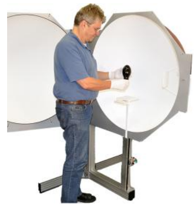
BTS256-LED Tester with 1m diameter integrating sphere
