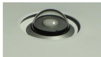
Entrance optic is blow-dried by warm air to prevent dirt, rain or snow
