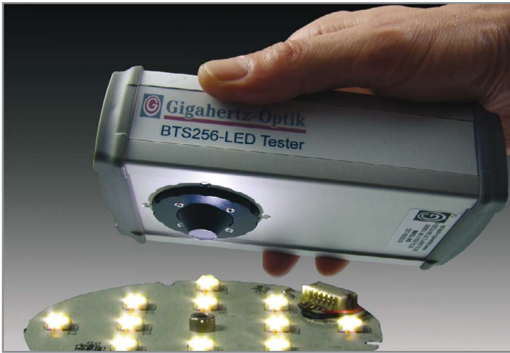
Figure 3: BiTec sensor technology enables compact size portable LED measurement devices with compact integrating spheres to measure luminous flux and color data of assembled single LEDs.
