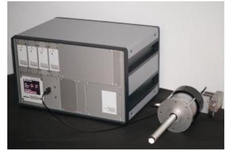
*Integrating sphere light source model ISS-8P-RVA-ROD with optional control electronic.*
