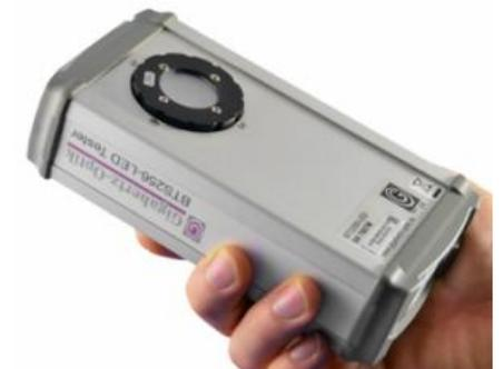
*BTS256-LED with the optional diffuser window for illuminance measurement*
