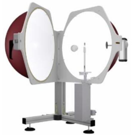
*BTS256-LED with an optional 50 cm diameter integrating sphere that has a sample holder for 4 $\pi$  lamps.*
