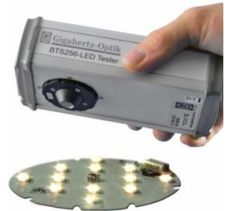
*BTS256-LED with the optional diffuser window for illuminance measurement*
