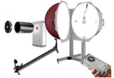
*BTS256-LED for measurement of the luminous flux, spectrum, color, and color rendering index of single LEDs*
