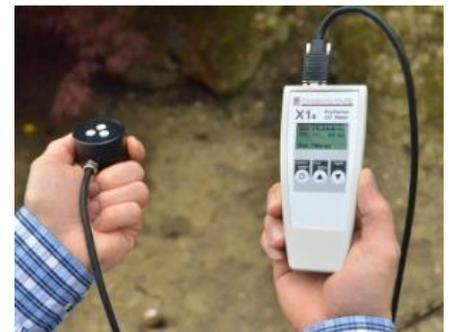
X14 being used for the measurement of UV radiation due to solar radiation.
