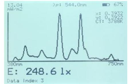
*Standard display with illuminance, x,y color coordinates, color temperature and emission spectrum of an energy saving lamp*
