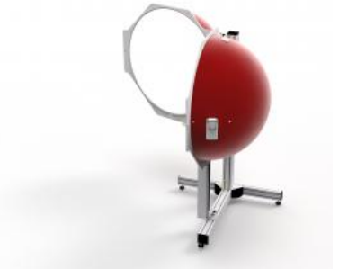
BTS256-LED spectroradiometer with integrating sphere ISD-100HF-V01 for 2pi and 4pi LED lamps inside the sphere. ISD-100HF-V02 with additional measurement port with plug.
