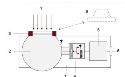
*1) BTS256-LED & BTS256.LED-DA 2) Integrating sphere 3) Precision bayonet mount with diffus window 4) BiTec sensor with Si photodiode, CMOS diode array spectrometer and shutter 5) Microprocessor 6) USB 2.0 interface 7) Light incident 8) Conical measurement port with precision bayonet mount*
