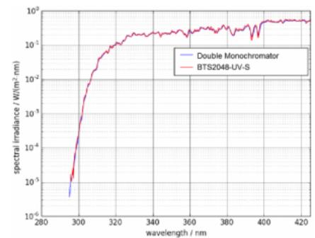
*Comparison of a solar measurement of the BTS2048-UV-S and a standard double monochromator. The BTS2048-UV-S achieves about the same quality in a measurement time of a few s compared to about 1.5 min of the double monochromator.*
