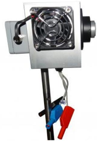
*Deuterium calibration standard for the UV range in 2Pi geometry*
