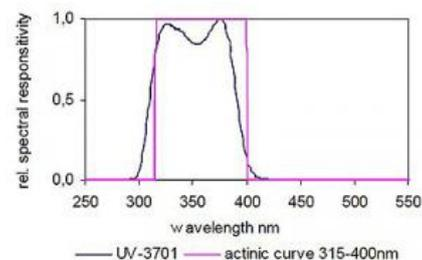
*UV-3701 UV-A Detector Typical Spectral Responsivity*
