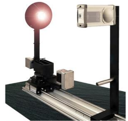
BTS256-LED Tester am GB-GB-360 Goniometer
